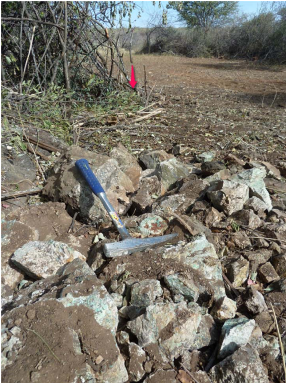
Figure 5 – Outcropping copper mineralisation broken up by track clearing, located directly behind planned drillhole indicated by red arrow at Deblin West Anomaly 1
