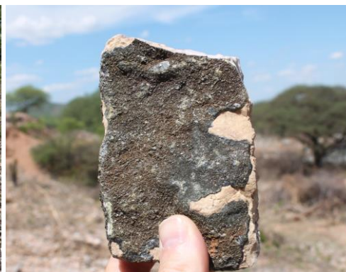
Dark vanadium bearing crust on a carbonate clast from the Abenab broken ore stockpile
