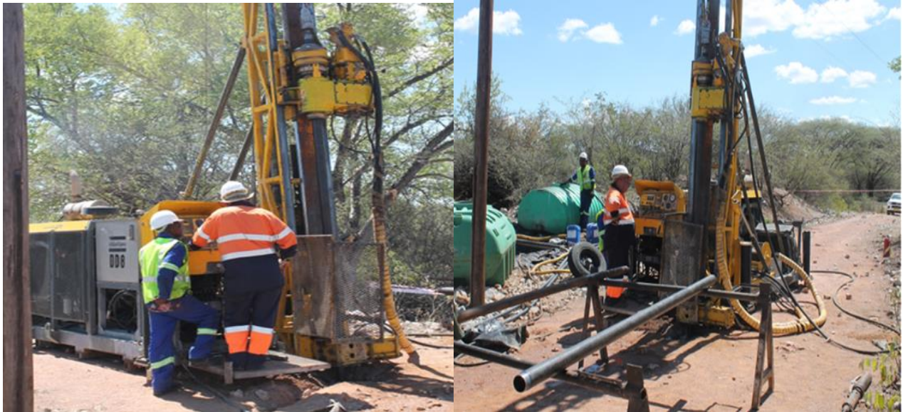
Figure 3-4: Diamond drilling at Abenab Mine.
