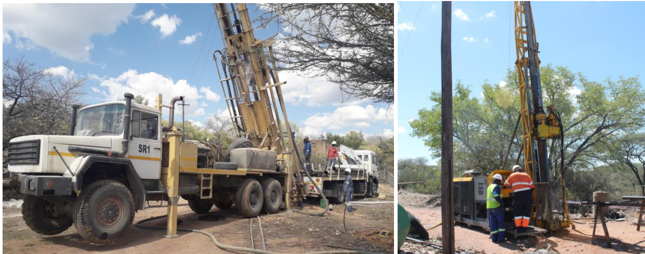
Figure 1-2: RC and diamond drill rigs in operation at the Abenab Mine.
